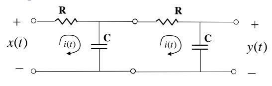
$$H(\omega) = \left(\frac{1}{1 + j\omega RC}\right)\left(\frac{1}{1 + j\omega RC}\right)$$
