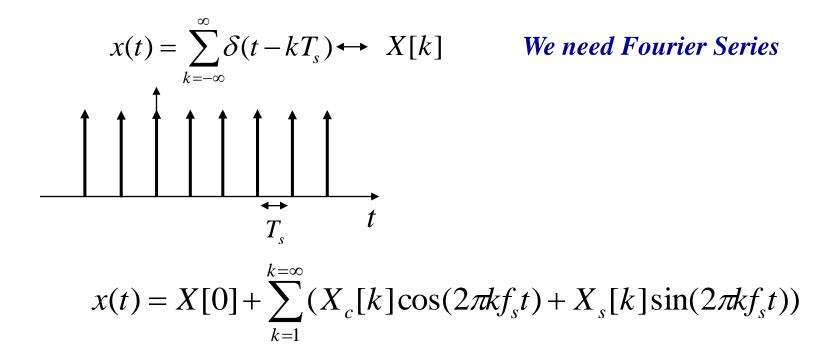
$$X[0] = \frac{1}{T_s} \int_{t_0}^{t_0 + T_s} x(t) dt = \frac{1}{T_s} \int_{0}^{T_s} \delta(t) dt = \frac{1}{T_s}$$
