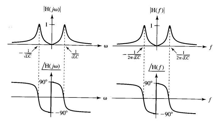
**Figure 6.36** Magnitude and phase frequency responses of a practical *RLC* bandpass filter.
