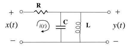
$$H(\omega) = \frac{j\omega/RC}{(j\omega)^2 + j(\omega/RC) + (1/LC)}$$
