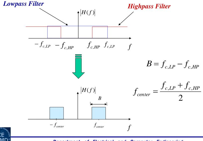
Lowpass and Highpass combined to generate Bandstop Filter
