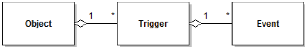
Figure 3.2: Duck’s event system. Every geometric object in a scene has zero or more triggers associated with it; every trigger has zero or more events associated with it. When a trigger fires, all of its associated events are executed.
