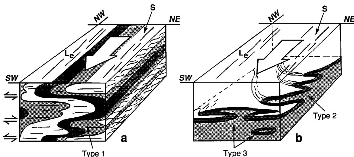
Fig. 4. Block diagrams summarizing different mesoscopic fold types relative to geometry of L-S tectonite fabrics. Open arrows show sense of ductile shear. (a) Open type 1 cylindrical folds with axes parallel to elongation lineation ( $L_e$ ) that signify minor  $L_e$ -normal strain during dominant  $L_e$ -parallel flow. (b) Asymmetric type 2 cylindrical folds with axes normal to  $L_e$ , which may evolve to noncylindrical type 3 sheath folds with noses parallel to  $L_e$  at high strains.
