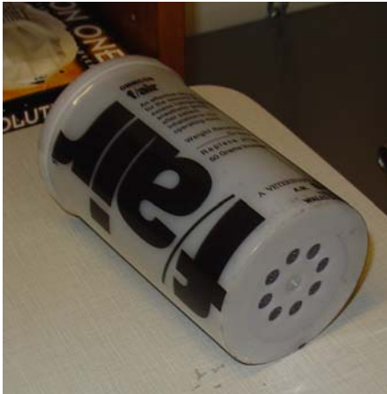
f/air gas scavenging canister with exhaust ports on the bottom
