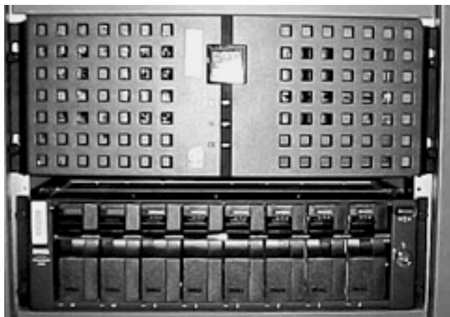
The new UMD_IS3 server, with dual CPUs and a 64Gigobyte RAID disk array.
