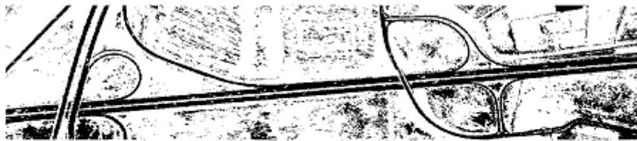
Figure 3.2 Binary image obtained after thresholding the image in figure 2.2.1 a)
