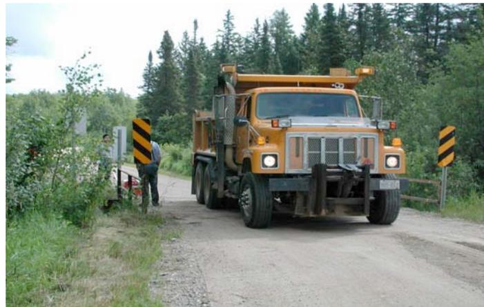
On July 13, 2005, bridge #726 in St. Louis County was similarly tested. This three-span bridge was constructed of 14 stringer beams covered by transverse running boards. Due to time constraints, only the middle and west spans were tested. The middle span was dead-load tested, as well as vibrationally tested both with and without a center load of 1000 lbs.
