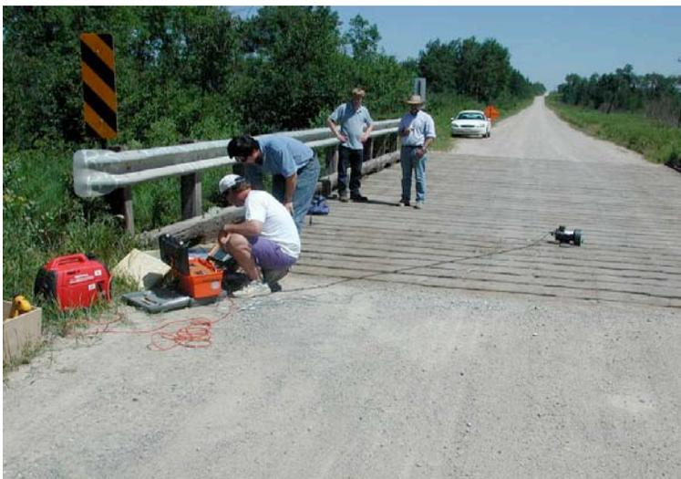
Dimensions of the middle span are 19.36 feet (length) and 24.35 feet (width.) Unloaded, the resonance frequency was observed to be 30.3 Hz, while under loading the resonance frequency was measured at 29.8 Hz. Thus in this test, bridge loading had a small affect on measured span resonance frequency. An estimate (using bridge component dimensions and an estimate of wood density) of span weight is 14,000 lb [39]. Thus, a 1000 lb load corresponds to
