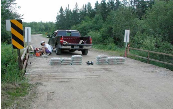
vibrationally both with and without a 1000 lb load placed center-span. This single-span bridge, is constructed of 13 stringers beams with a transverse plank surface. It has dimensions 17.9 feet (Length,  $L$ ) and 18.1 feet (width.) The observed resonance frequency for the unloaded span was 22.22 Hz, while the resonance frequency of the loaded span was measured at 26.46 Hz. The general theoretical framework described in [61] predicts that fundamental (bending) mode frequency should
