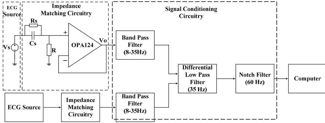
Fig. 4. ECG measurement circuitry for electrodes on backrest
