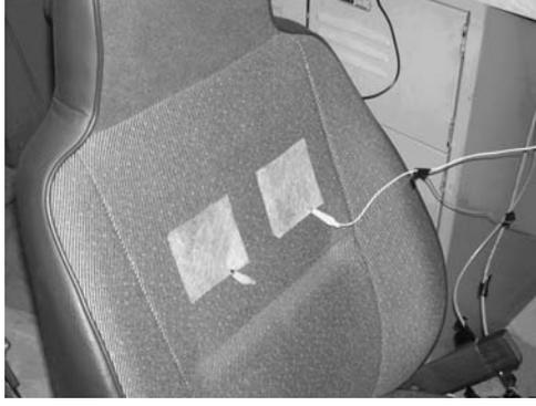
Fig. 3. ECG measurements on driver's seatback
