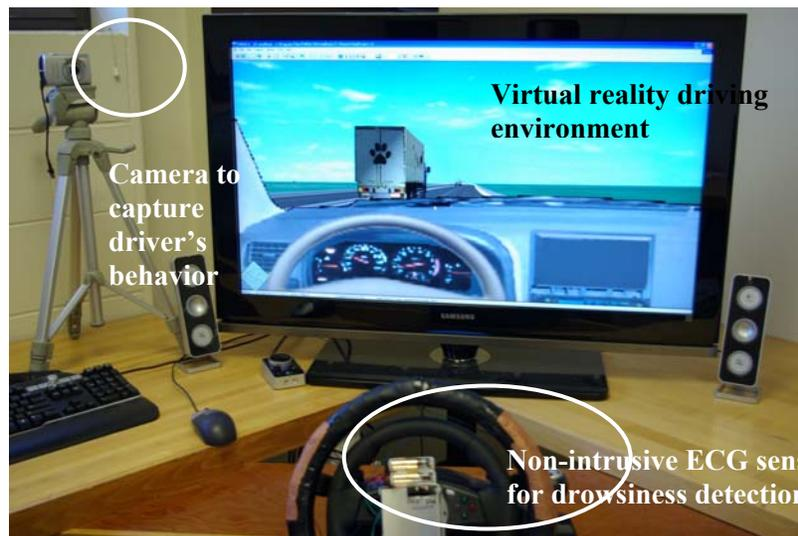
Fig. 11. Layout of driving simulator
