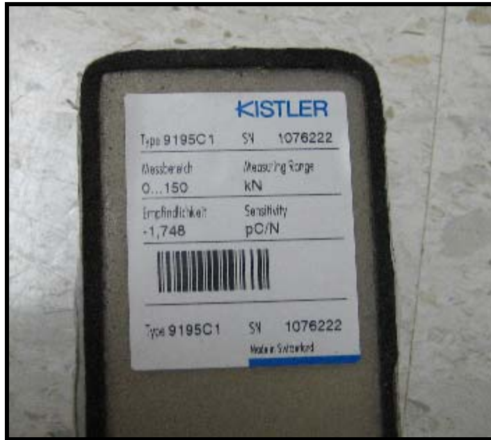
Figure 6.7: Factory sensitivity setting specified on the sensor
