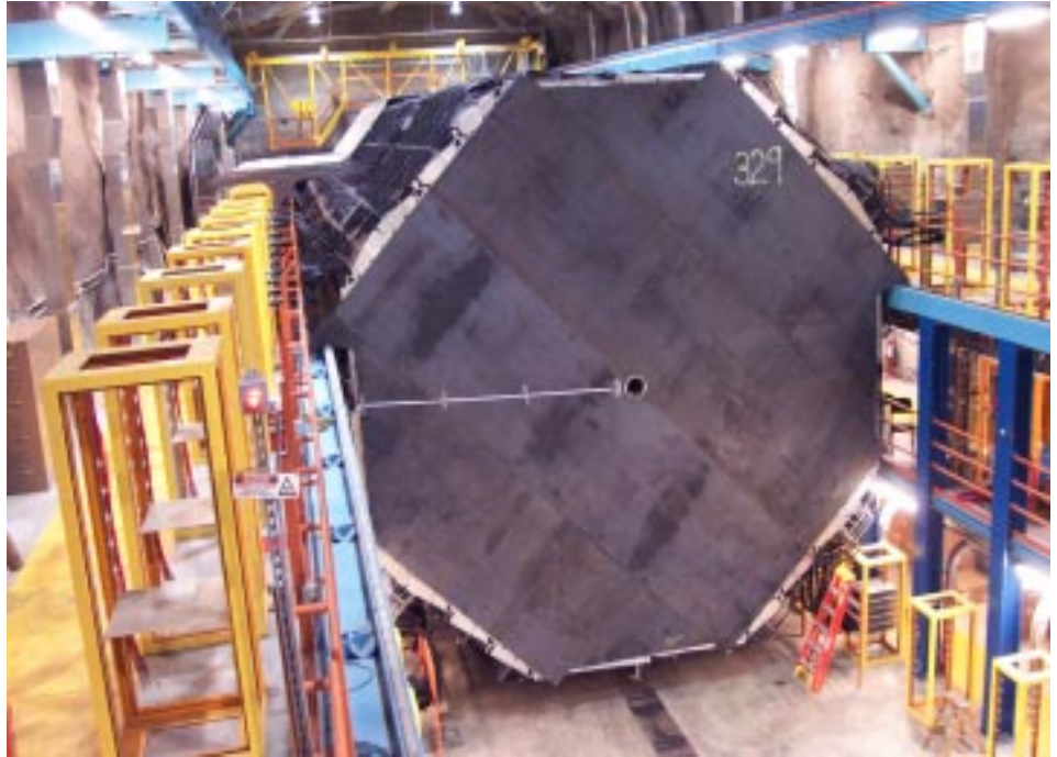
The MINOS far detector nearing completion. Slabs of steel alternate with scintillator in a sideways stack aligned with the neutrino beam to come from Fermilab, near Chicago. (photo by Jerry Meier, Sudan Underground Lab)
