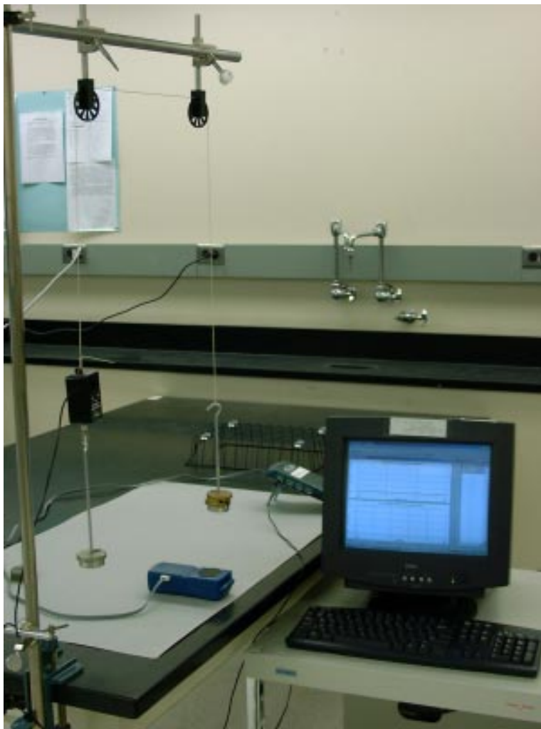
Experimental setup for "Atwood's Machine," using Vernier Logger Pro Software and motion and force sensors.
