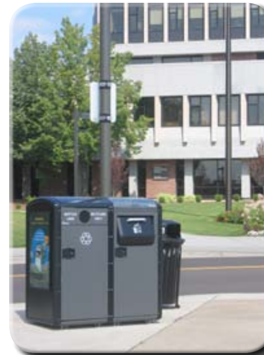
The BigBelly solar compactors found around campus reduce trash pickups, keep the birds and the bees out of the trash, and offer a place for outdoor recycling
