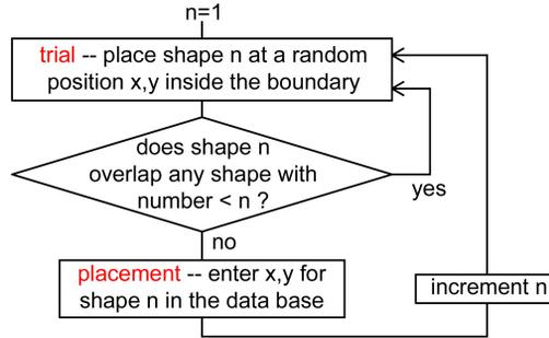
**Figure 2:** Flow-chart for non-overlapping random search, with definitions of what is meant by trial and placement.
