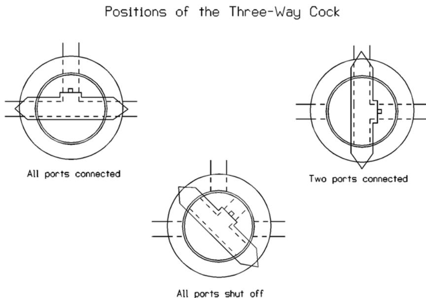
**Figure 2.** Three-way stopcock positions
