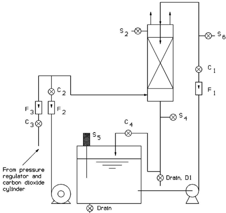
**Figure 1.** Gas Absorption Column System
