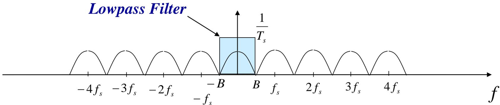
*bandwidth of lowpass filter = B Hz*
