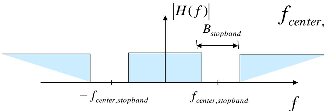
$$f_{center,stopband} = \frac{f_{c,LP} + f_{c,HP}}{2}$$
