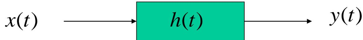
*$h(t)$  - Impulse Response of a Linear Time Invariant System*
