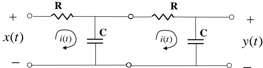
$$H(\omega) = \left(\frac{1}{1 + j\omega RC}\right)\left(\frac{1}{1 + j\omega RC}\right)$$
