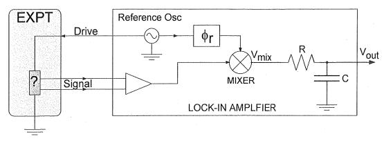
The reference oscillator provides the drive signal to the experiment and a replica of itself that has a fixed amplitude and user-adjustable phase shift  $\phi_r$  to the mixer. We'll assume for simplicity that the amplitude is simply 1.0 (volts) and the adjustable reference phase shift is  $\phi_r = 0$ , so  $V_r(t) = 1\cos(\omega_r t)$ .
