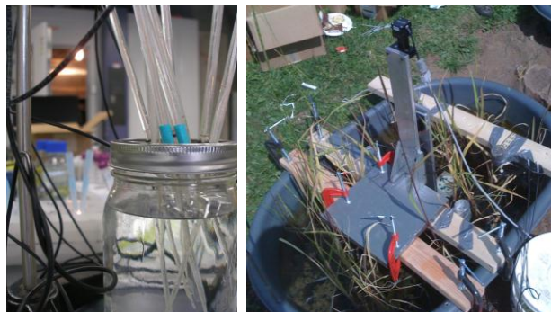
Figure 3. Microelectrodes fabricated in the lab and micropositioner deployed in Pastor's microcosm
