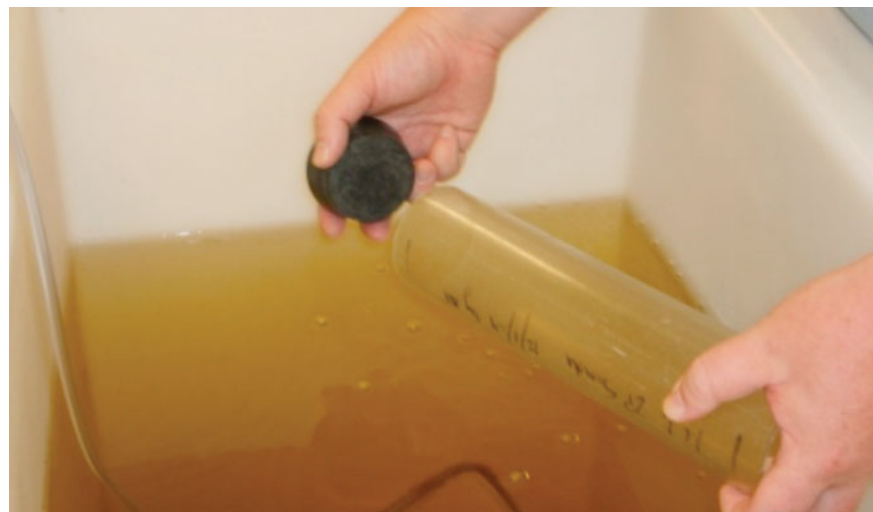
Image of a 230-L mesocosm tank partially filled with harbor water and a scientist holding a sampling tube used to retrieve zooplankton during routine, weekly monitoring of the tank.
