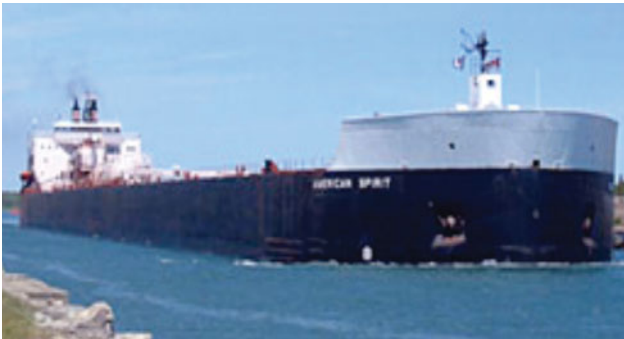
Figure 2: The M/V American Spirit is a cargo ship operating on the Great Lakes. L = 306 m, w = 32 m and midsummer draft 8.8 m (picture from American Steamship Company's web page).
