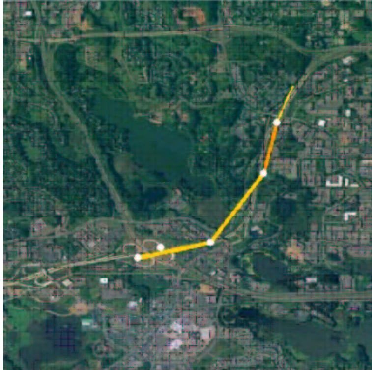
Figure 3.2: Map Visualization. This figure shows an example of map visualization. It shows the traffic on the sensors on northbound trunk highway number 212 on Friday evenings of January, 2002. The volume between the sensors is represented by the thickness of the line and the occupancy is represented by the color. Red color indicates high occupancy and yellow color indicates moderate occupancy. This visualization technique gives spatial information about the traffic to allow better comprehension of traffic flow on highways.
