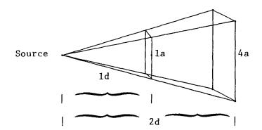
If the distance is doubled (2d:1d), the radiant energy covers 4 times the area (4a:1a). If d = 4, then a = 16. It is easy to see that the radiant energy from one square cm of the sun's surface is very much spread out by the time it reaches the earth 93,000,000 miles away.
