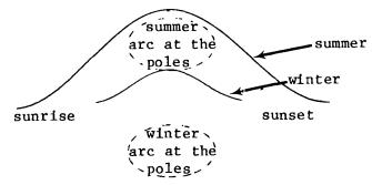
Solar energy flux on a clear day increases from sunrise to solar noon and decreases from solar noon to sunset. The pattern is nearly symmetrical about solar noon for a horizontal plane at the earth's surface, as illustrated by the tracing of two daily pyranometer recordings below.
