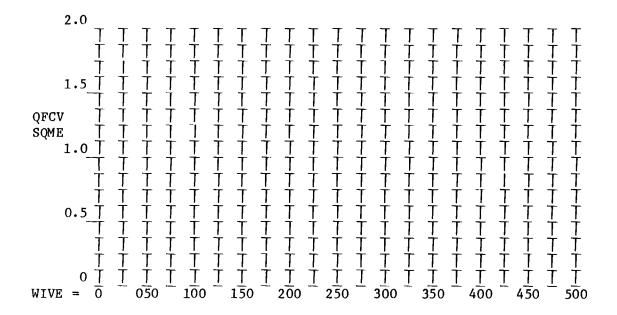
The results, expressed as the quantity of forced convection (QFCV) per square meter (SQME) is really a convection coefficient, an expression of the efficiency of heat transfer with various combinations of wind velocity and cylinder diameter This coefficient may be multiplied by DLTA and SAFC to determine the absolute amount of heat lost by forced convection from a defined surface.
