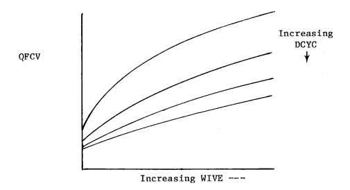
Temperature differences. When wind velocities and the characteristic dimensions of the convectors remain constant, the amount of heat loss per unit surface area is directly proportional to the temperature differences. This is obvious from the formula; DLTA functions as a simple multiplier after the non-linear effects of WIVE and DCYC or LFPC have been considered. The effects of temperature differences are illustrated below.
