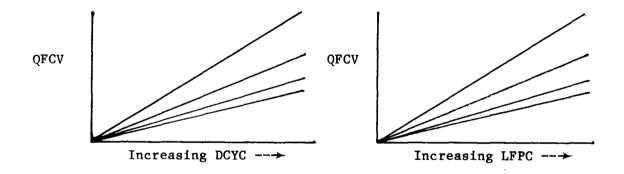
The smaller the diameter of the cylindrical convector or the length of a flat plate convector, the greater the sensitivity to changes in WIVE. Efficiency of heat loss is associated with small-diameter convectors and short plates. The non-linear characteristic of this relationship is clear.
