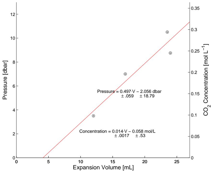
Figure 4.13: Calibration of 4 mm ID/7 mm OD silicone tubes from in pressure chamber with CO<sub>2</sub> saturated water. The vertical axes show gas pressure above the water and the estimated molar concentrations of CO<sub>2</sub> in the water.
