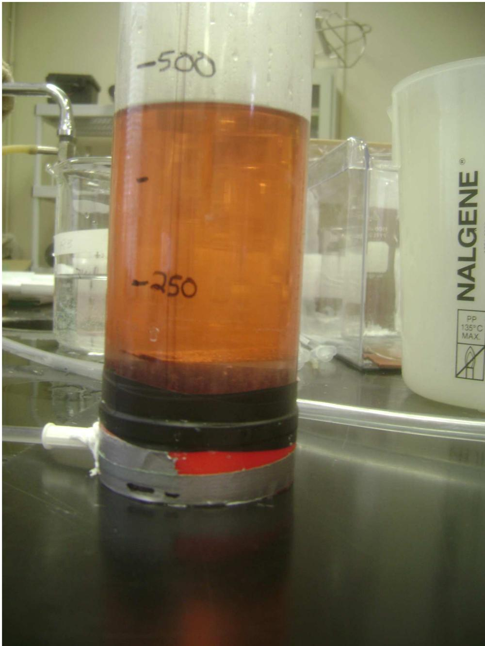
Figure 3.10: View of the bottom half of the tall narrower tube used to replace the beaker initially used in attempts to create a small scale limnic eruption.
