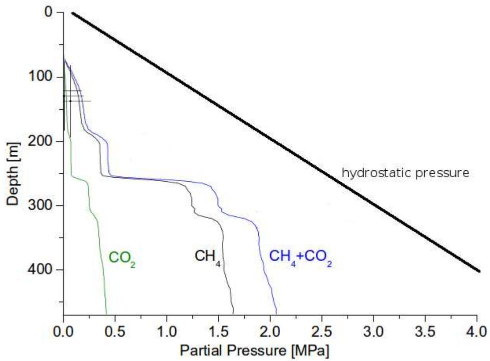
Figure 4.14: Fitting of the silicone tube estimated pressures onto the partial pressures of Figure 5 produced by Schmid et al. (2002).
