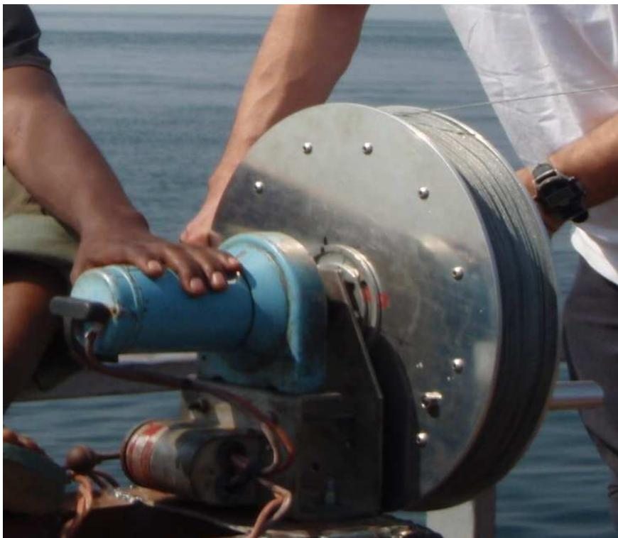
Figure 3.3: Picture of the winch used to raise and lower the CTD profiler (primarily by hand) through the water column in January 2011.
