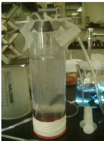
Figure 3.9: Image of the bubble chamber created to dissolve CO<sub>2</sub> into the water prior to drip-feeding the water into the lower layer of the beaker or the narrow tube which replaced the beaker
