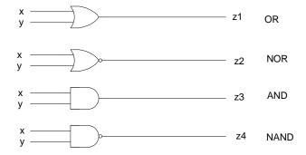
Remember to connect the power supply **Vcc** and **GND** lines to the TTL chip. Also, remember that any outputs of the gate cannot be connected together. If you do so, it causes a short circuit and will destroy the chip or the LogiScan interface.
