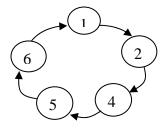
For the T-ff function, use 74LS76 (JK-ff) by connecting the J and K inputs together. 74LS76 chips contain two JK-ffs, and each JK-ff has Preset and Clear control inputs that work active low, so both pairs of Preset and Clear should be tied to +5V for normal FF operations. Also, be careful in connecting Vcc and GND. Vcc is at Pin 5 and GND is at Pin 13 in 74LS76. Since the states are the outputs of your circuit (counter), connect the three states to LogiScan F0, F1 and F2, and test the counter.
