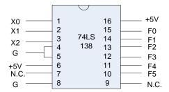
After learning about the 74LS138 chip, build the circuit for the given functions g(x,y,z) and h(x,y,z) on your breadboard and verify your circuit using LogiScan. Fill in the truth table observed from the LogiScan.
