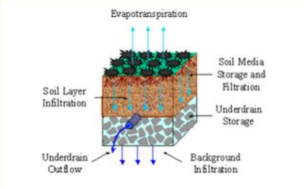
Figure 3-10. Processes considered in an underdrain structure.
