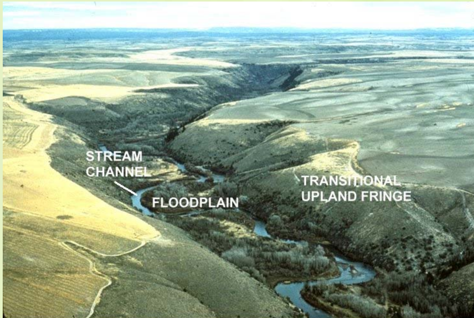
Fig. 1.10a -- The three major components of a stream corridor in different settings. In Stream Corridor Restoration: Principles, Processes, and Practices, 10/98 by the Federal Interagency Stream Restoration Working Group (15 Federal Agencies of the US)
