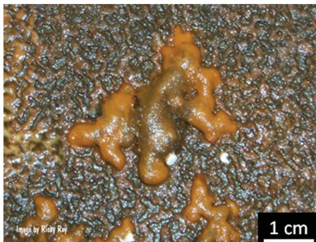
**Figure 2.** Tubercle on carbon steel after 1-year exposure in DSH
