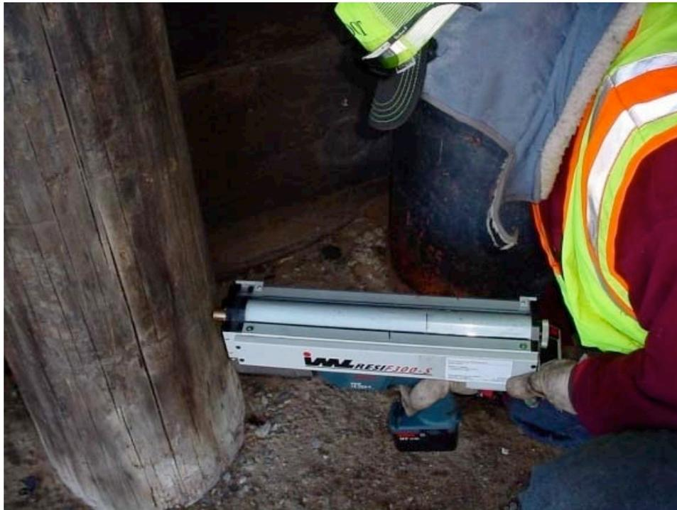
**Figure 3.2.** Example of resistance drill testing.
