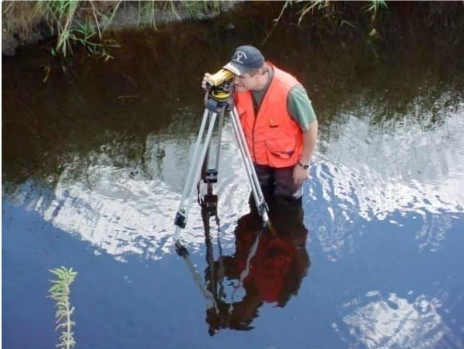
**Figure 3.6.** Optical surveying level.
