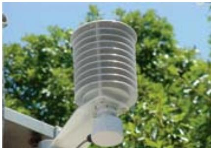
**Figure 2.5: Air Temperature and Relative Humidity Sensor**
