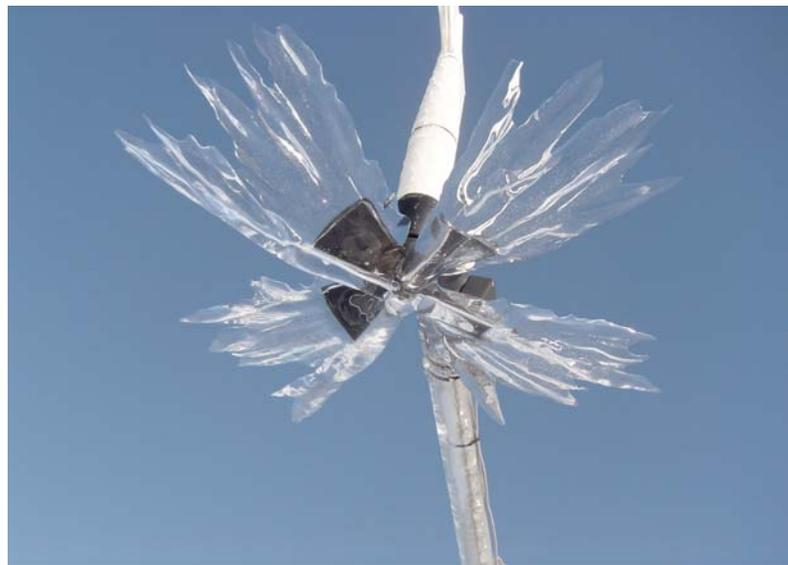
**Figure 2.14: Ice Accumulated on the blades of Wind Sensor**
