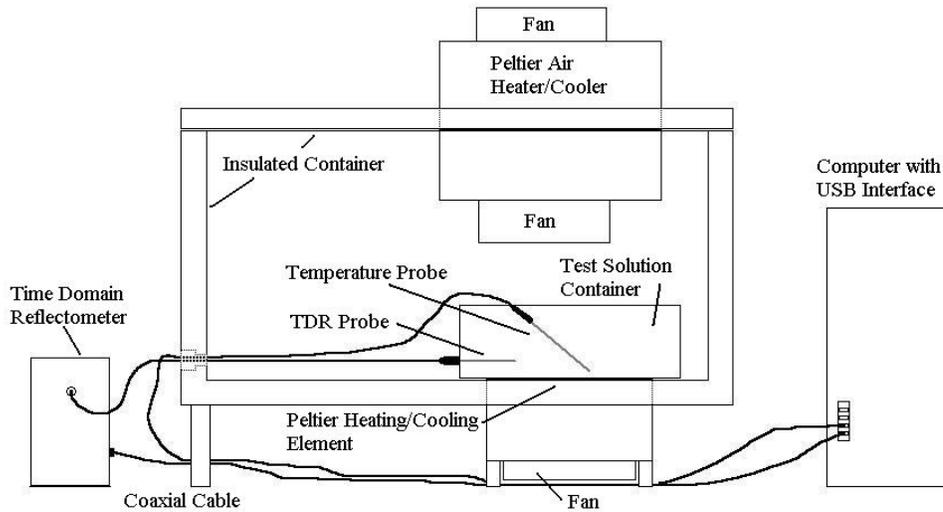
Figure 3.1 Block diagram of temperature controlled test cell.
