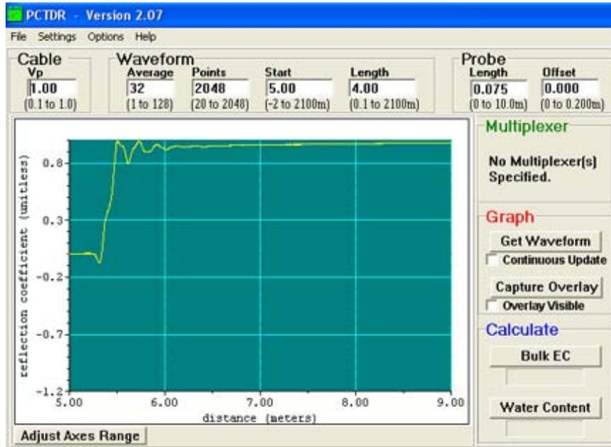
Figure 5.2. PCTDR program interface with air waveform displayed.
