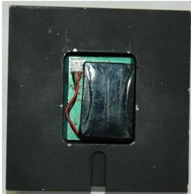
**Figure 17: Wireless node inside a sensor housing.**
