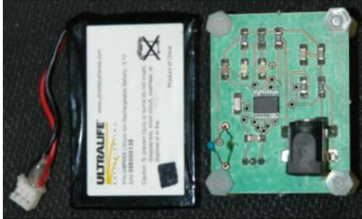
Figure 14: Battery charger circuit and li-ion rechargeable battery.
