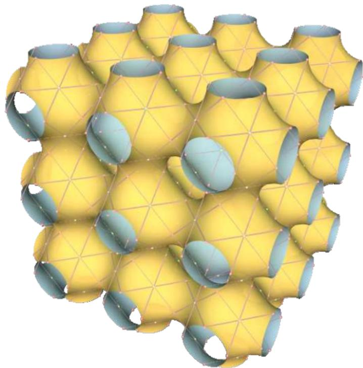
**A close-up of Schwarz's P-surface showing corresponding embedded lines and "skew rhombi"**
