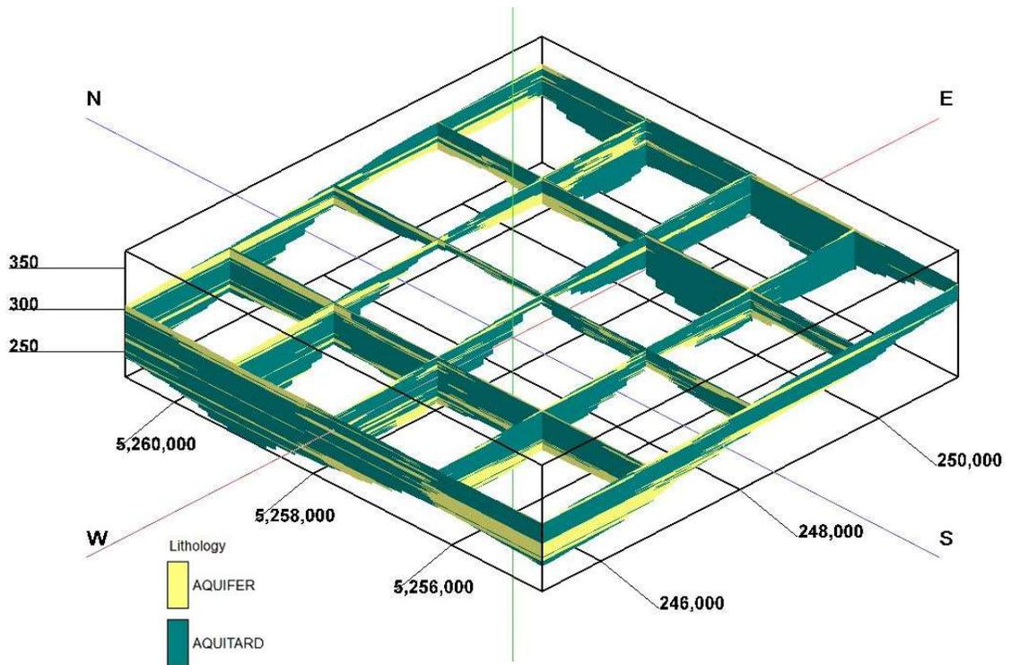
Figure 43. Fence diagram of stratigraphy in immediate area around Agassiz-Nelson Fen. Agassiz-Nelson Fen is located at the center. Vertical exaggeration 10x. Units in meters. Horizontal values are UTM Zone 15N Extended.
