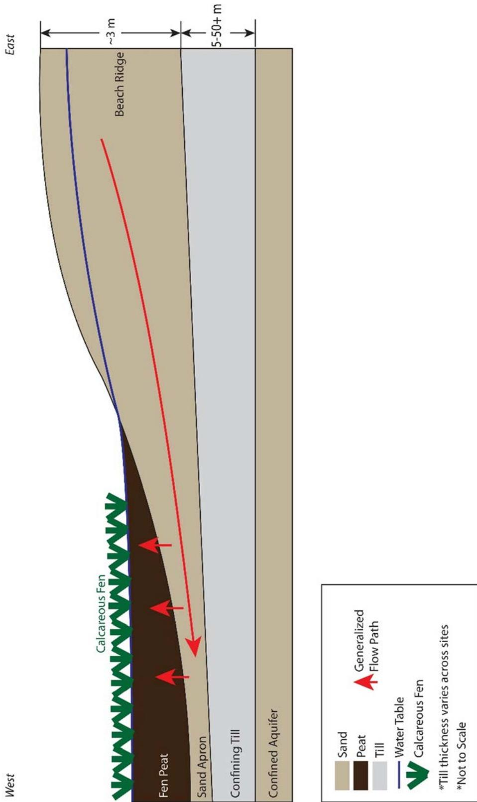
Figure 46. Hydrology of Beach Ridge Calcareous Fens. Arrows are generalized water flow paths.
