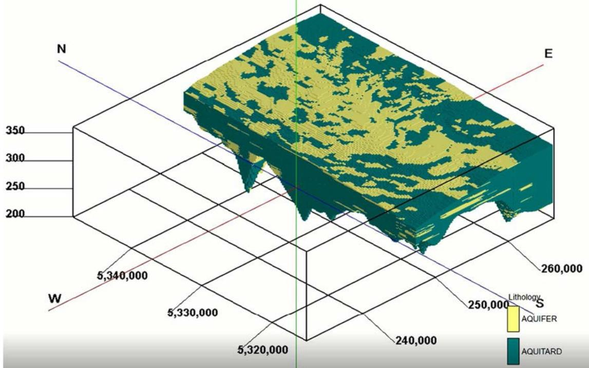
Figure 38. North-south cross-section through Sanders Fen Rockworks 3D model. Sanders Fen is located at the intersection of the axis lines. Vertical exaggeration 64x. Units in meters. Horizontal values are UTM Zone 15N Extended.
