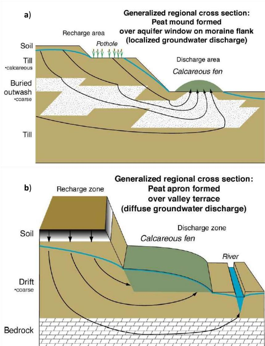
Figure 2. MNDNR conceptual models of calcareous fen hydrology including groundwater flow paths for **a)** a morainal aquifer window setting and **b)** a river valley terrace setting (MNDNR, 2017).
