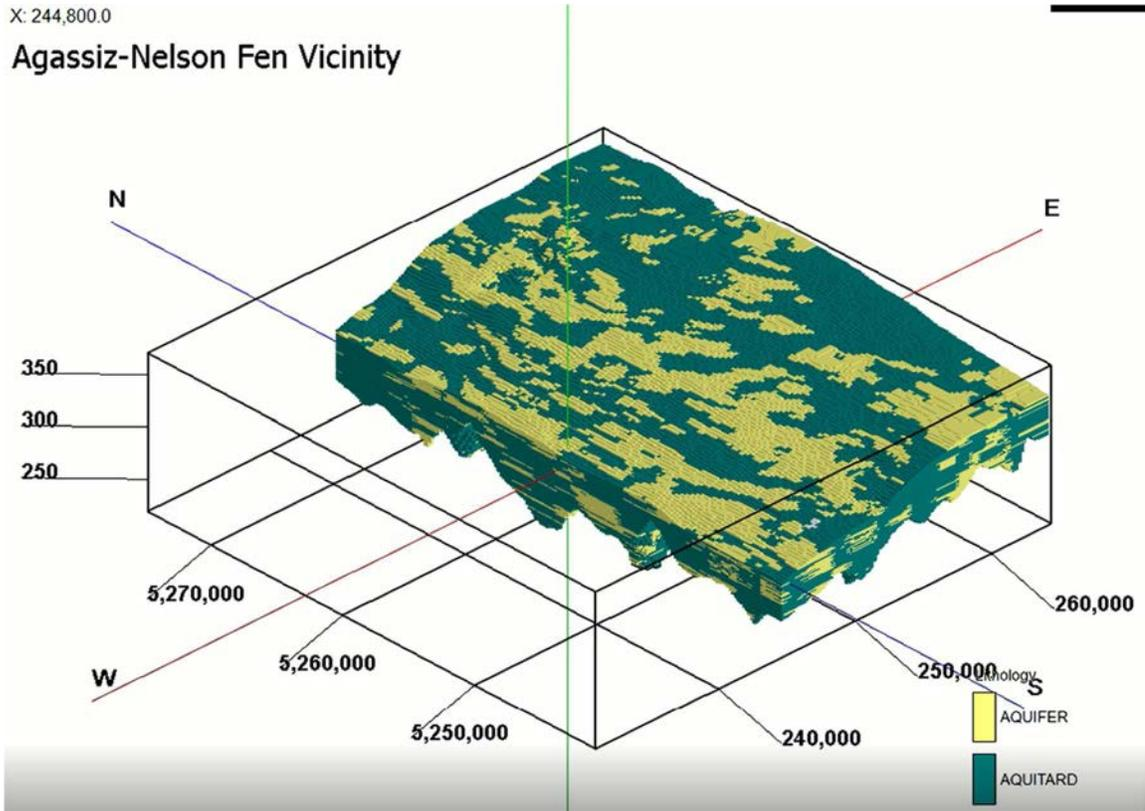
Figure 40. North-south cross-section through Agassiz-Nelson Fen Rockworks 3D model. Agassiz-Nelson Fen is located at the intersection of the axis lines. Vertical exaggeration 64x. Units in meters. Horizontal values are UTM Zone 15N Extended.
