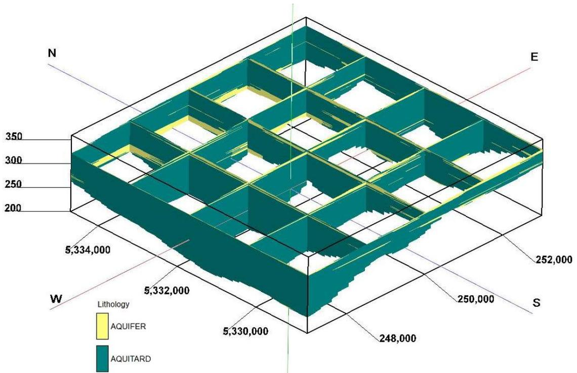
Figure 42. Fence diagram of stratigraphy in immediate area around Sanders Fen. Sanders Fen is located at the center. Vertical exaggeration 10x. Units in meters. Horizontal values are UTM Zone 15N Extended.
