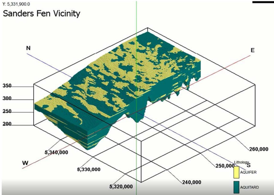
Figure 39. East-west cross-section through Sanders Fen Rockworks 3D model. Sanders Fen is located at the intersection of the axis lines. Vertical exaggeration 64x. Units in meters. Horizontal values are UTM Zone 15N Extended.
