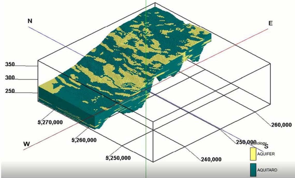
Figure 41. East-west cross-section through Agassiz-Nelson Fen Rockworks 3D model. Agassiz-Nelson Fen is located at the intersection of the axis lines. Vertical exaggeration 64x. Units in meters. Horizontal values are UTM Zone 15N Extended.
