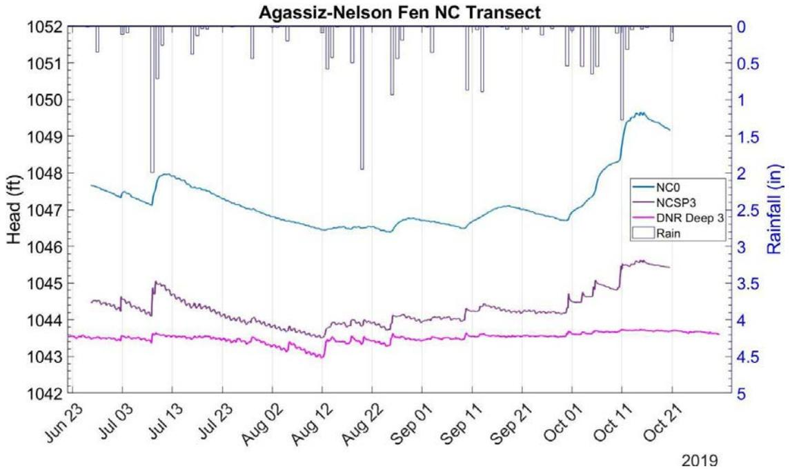
Figure 14. Agassiz-Nelson Fen NC transect hydrograph with rainfall at Twin Valley, MN. DNR Deep 3 well is also included on this figure because of the spotty record of well NN3.
