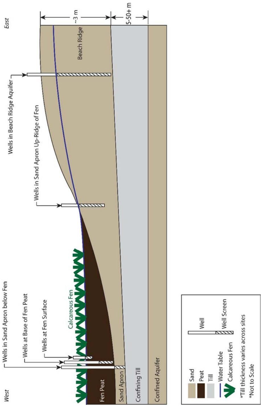
Figure 5. Typical cross section of a calcareous fen and beach ridge and the locations of surficial system wells.
