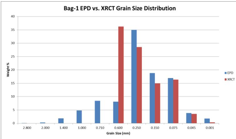
**Figure 5.99** Grain size distribution comparison of EPD and XRCT material from sample Bag-1. The EPD data does still contain silicate material whereas the XRCT data only contains ore grain information.
