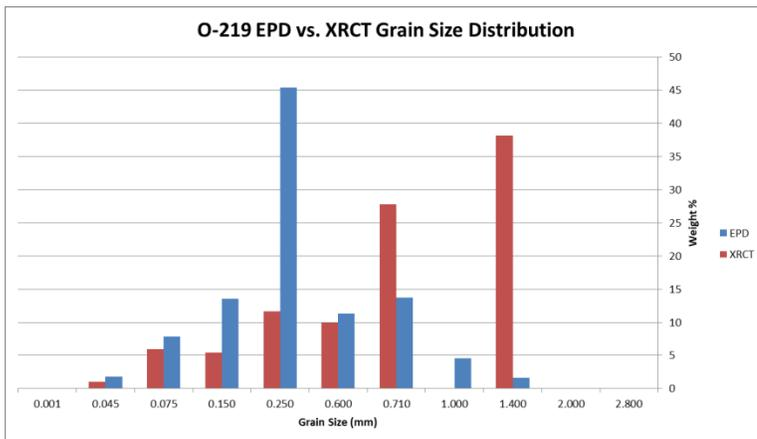
**Figure 5.101** Grain size distribution comparison of EPD and XRCT material from sample O-219. The EPD data does still contain silicate material whereas the XRCT data only contains ore grain information.
