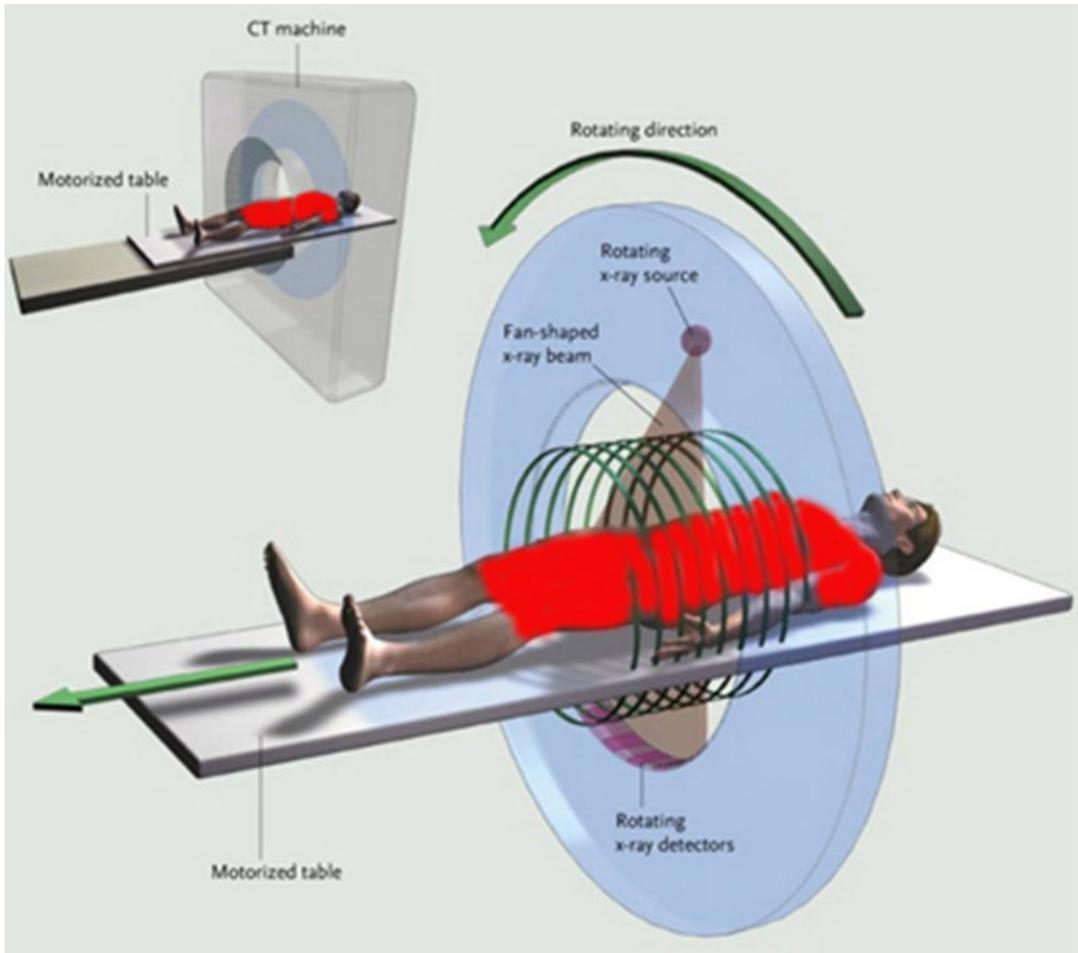
**Figure 4.3** A schematic diagram illustrating the basic parts and functions of a medical CT scanner (Brenner and Hall, 2007)
