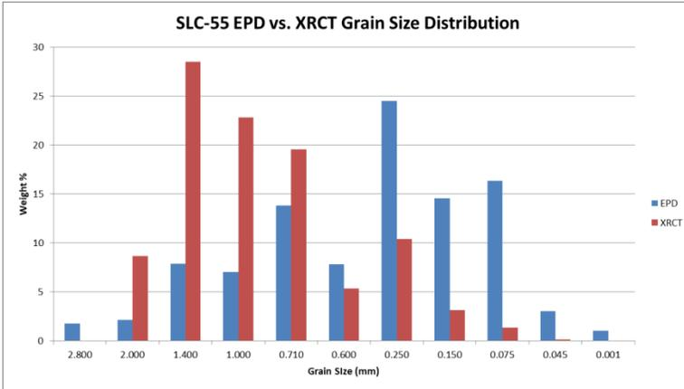
**Figure 5.102** Grain size distribution comparison of EPD and XRCT material from sample SLC-55. The EPD data does still contain silicate material whereas the XRCT data only contains ore grain information.
