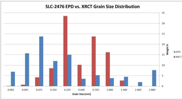
**Figure 5.103** Grain size distribution comparison of EPD and XRCT material from sample SLC-2476. The EPD data does still contain silicate material whereas the XRCT data only contains ore grain information.
