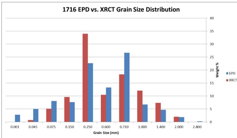
**Figure 5.105** Grain size distribution comparison of EPD and XRCT material from sample 1716. The EPD data does still contain silicate material whereas the XRCT data only contains ore grain information.
