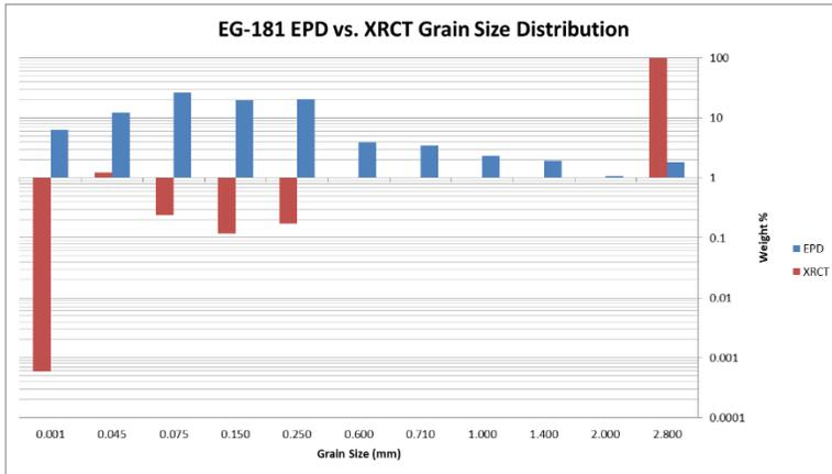
**Figure 5.96** Grain size distribution comparison of EPD and XRCT material from sample EG-181. The EPD data does still contain silicate material whereas the XRCT data only contains ore grain information.
