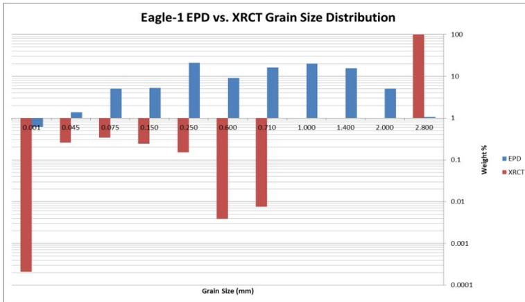
**Figure 5.97** Grain size distribution comparison of EPD and XRCT material from sample Eagle-1. The EPD data does still contain silicate material whereas the XRCT data only contains ore grain information.
