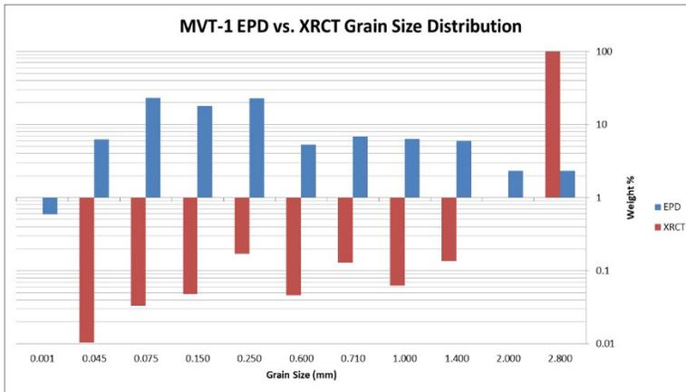
**Figure 5.104** Grain size distribution comparison of EPD and XRCT material from sample MVT-1. The EPD data does still contain silicate material whereas the XRCT data only contains ore grain information.
