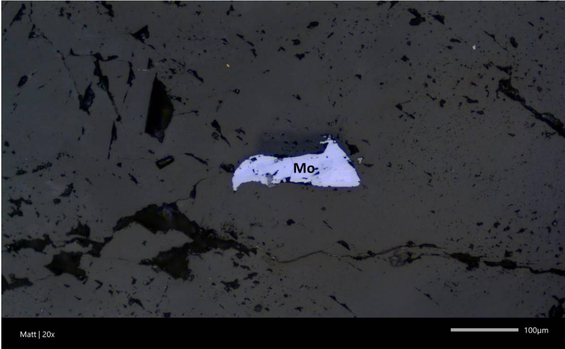
**Figure 5.16** Sample O-219 at 20x magnification, molybdenite (Mo) reflectance is a medium to blueish-grey color, anhedral, strong bireflectance.
