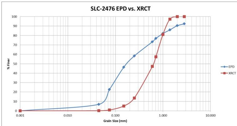
**Figure 5.93** Sieve analysis comparison of EPD and XRCT material from sample SLC-2476.
