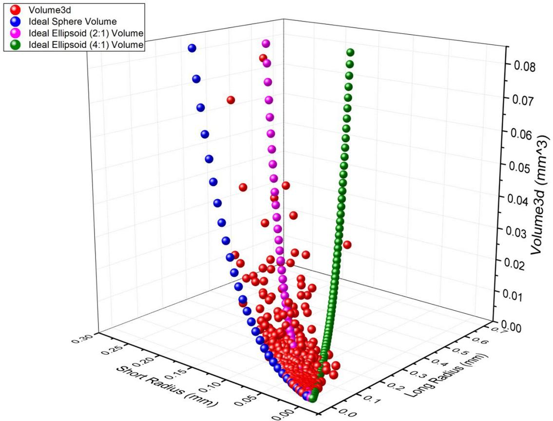
**Figure 5.66** Shape analysis graph plotting the long and short radius against the 3D volume for sample Eagle-1. Ideal shape distributions appear as the blue, pink, and green data points.
