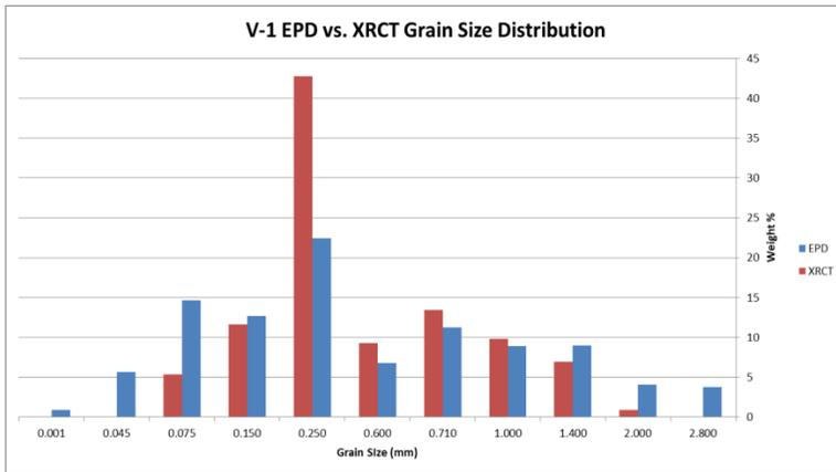
**Figure 5.100** Grain size distribution comparison of EPD and XRCT material from sample V-1. The EPD data does still contain silicate material whereas the XRCT data only contains ore grain information.
