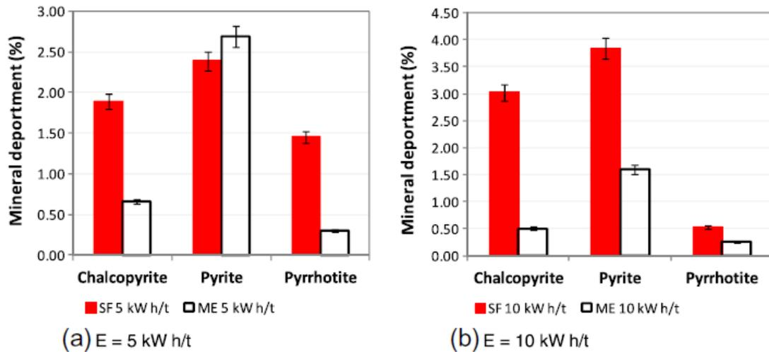
**Figure 6.3** Greater than 95% liberation values for the indicator minerals for 3 different ore samples that were processed using two different specific energy levels. White bars represent material that was mechanically comminuted while the red bars represent material that was comminuted in an EPD, error bars represent 95% confidence interval (Wang et al., 2012a).
