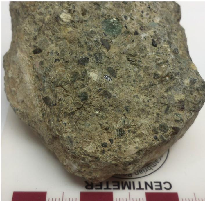
Figure 9.22 Hand sample photo for Lake Ellen Kimberlite.
