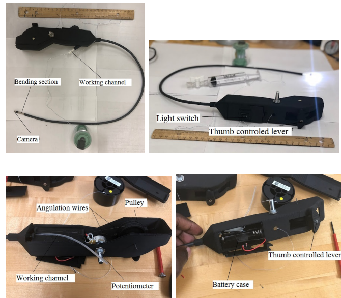
Figure 5: Top left and top right: working mechanical prototype. Bottom left and bottom right: open prototype handle.
