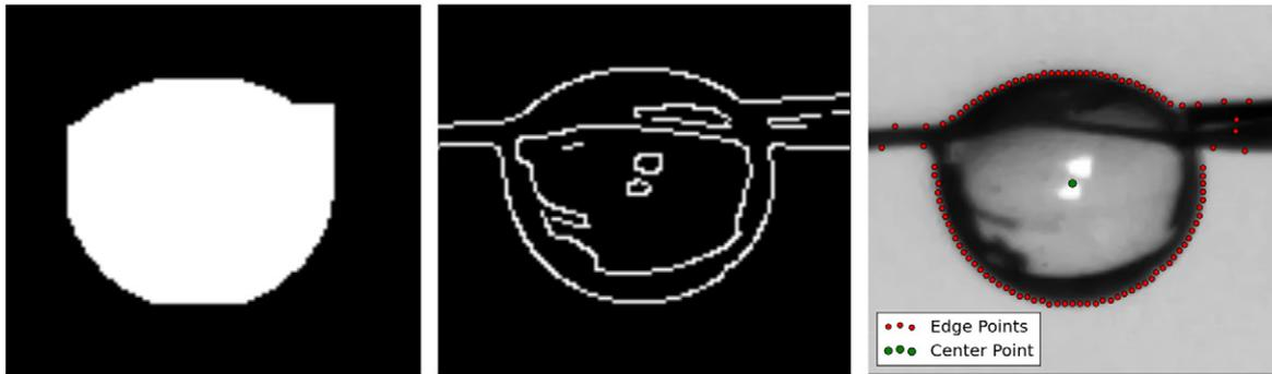
Figure 12. Detected binary droplet region (left), Canny edge image of the droplet (center), and edge points used for curve fitting (right).
