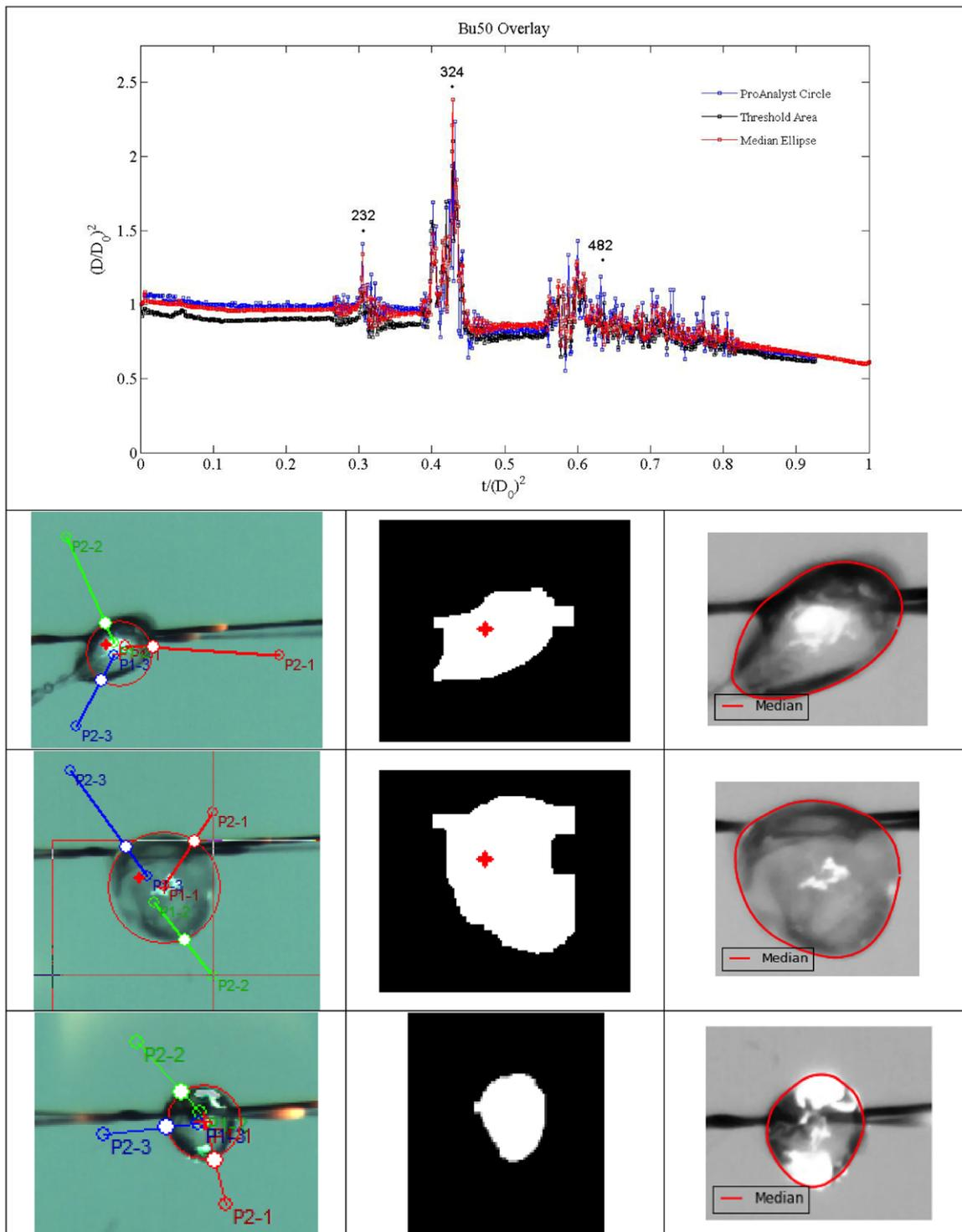
**Figure 15.** The left column shows the previous method used to quantify droplet size using the ProAnalyst commercial software package, the middle column shows the morphological area obtained using ProAnalyst, and the right column shows the contour obtained using the proposed median ellipse parameterization algorithm.
