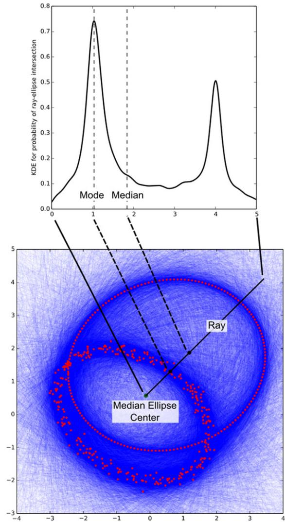
Figure 8. The ellipse cloud used to generate the fit shown in figure 7 is shown at the bottom. The kernel density estimation along a single ray is shown at the top with the median and mode locations indicated by vertical lines.
