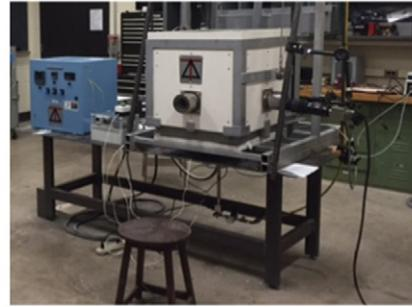
**Figure 9.** Droplet combustion experimental facility. A schematic is shown on the left and a photograph of the actual setup is shown on the right.
