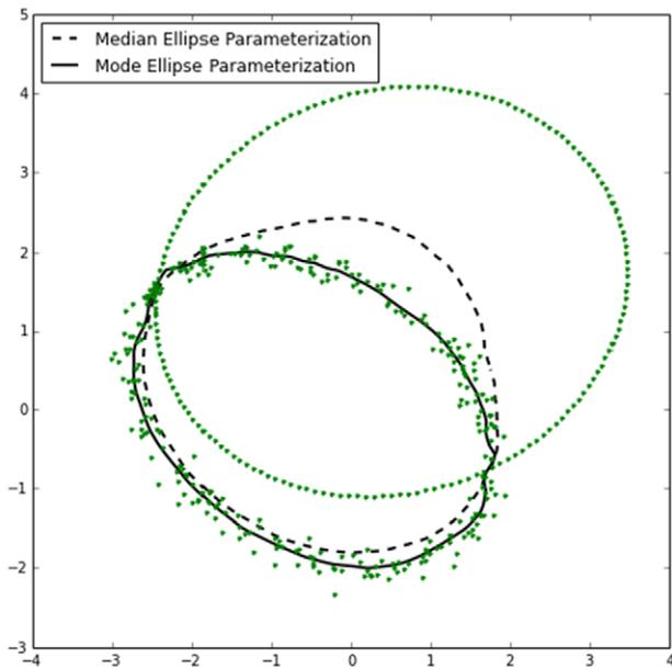
Figure 7. Median ellipse parameterization applied to an example with an increased number of outliers.
