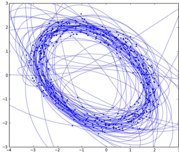
Figure 1. Ellipses fitted to subsets of five points.
