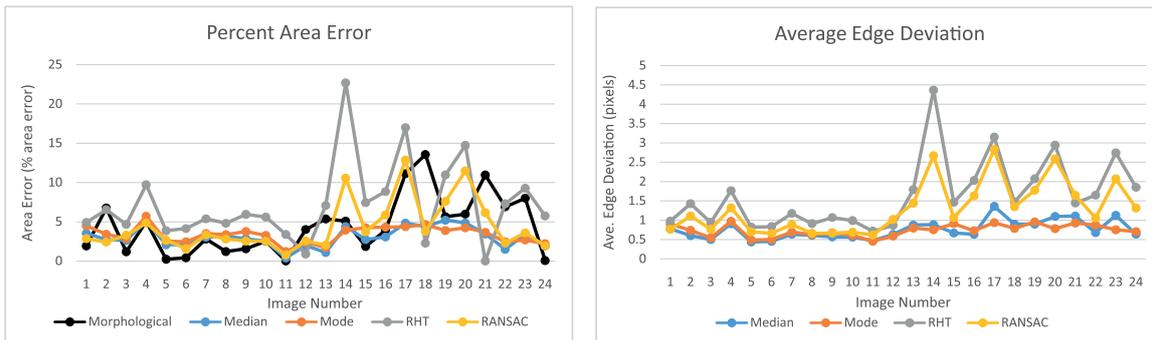
**Figure 14.** Fitting error for the robust contour fitting algorithms evaluated.
