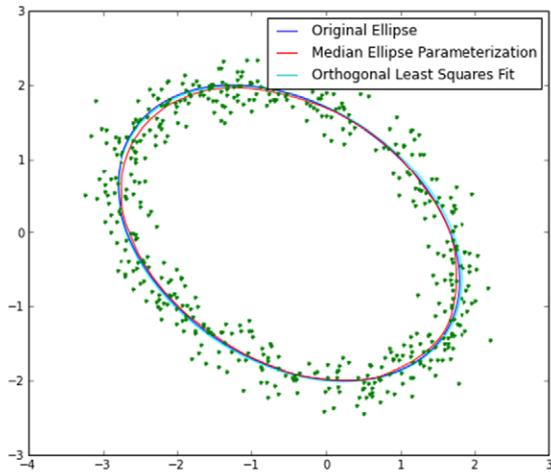
Figure 3. Noisy ellipse shown with original ellipse, orthogonal least squares fit, and the median ellipse fit.
