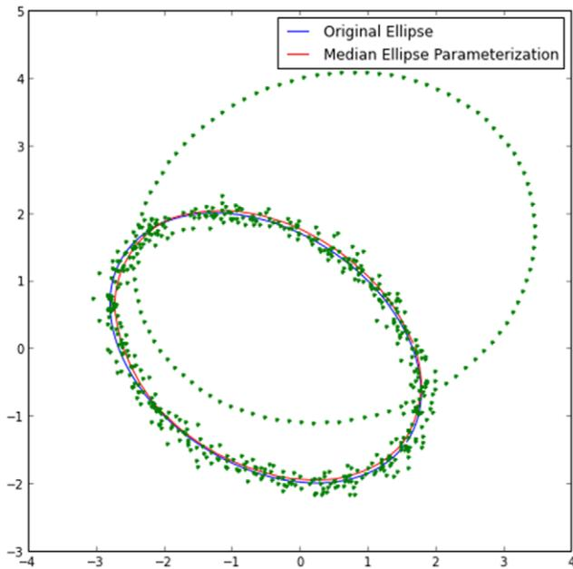
Figure 6. Median ellipse parameterization applied to an example with outliers.
