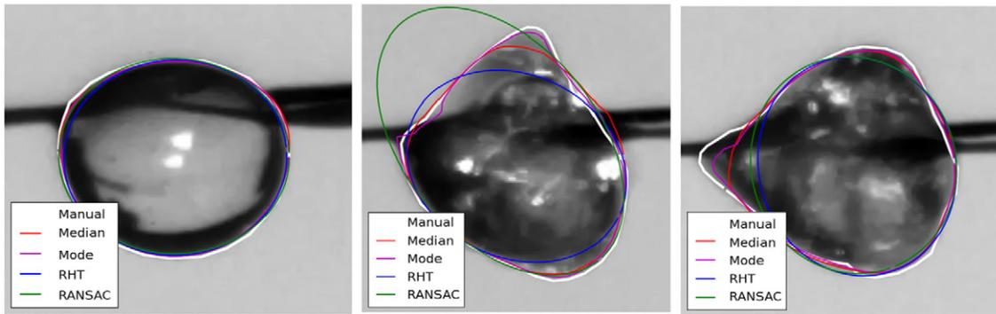
**Figure 13.** Three frames from the droplet combustion image sequence with curve fits. Droplet before microexplosions on the left and droplet after the initiation of microexplosions at the center and right.
