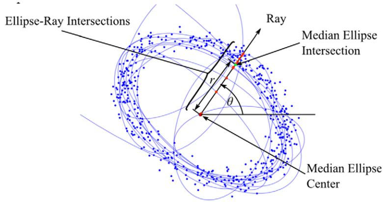
Figure 2. Calculation of curve fit radius based on the median intersection of the ellipse fits.
