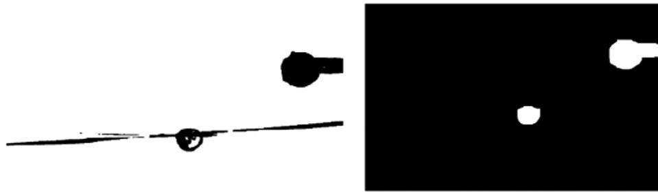
Figure 11. Otsu threshold image on left. Image after morphological operations on right.
