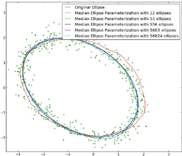
Figure 5. Impact of the number of ellipses on the median curve fit.
