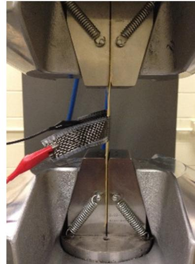
**Figure 4.** Experimental setup for tensile test.
