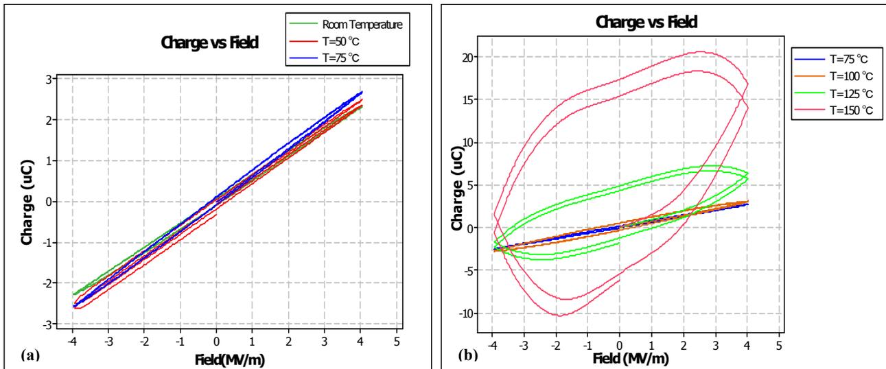
Figure 11. Comparison of the hysteresis loop at T=75 °C with (a) hysteresis loops obtained at lower temperatures, (b) hysteresis loops obtained at higher temperatures.
