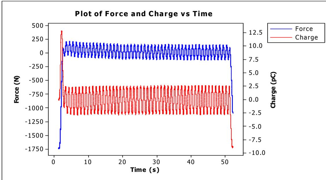
Figure 12. Plot of the charge generated in the sample poled at  $T=75^{\circ}\text{C}$  by applying 2000V for 20 minutes, due to an applied force in tensile test.
