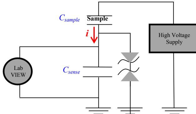
Figure 4. Schematic of the circuit used for generating hysteresis plots (P-E loops).
