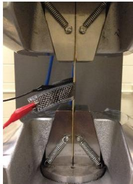
Figure 5. Experiment setting for tensile test.
