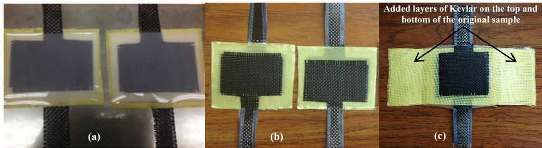
Figure 3. Prepared samples (a) original samples before melting the PVDF films, (b) original samples after melting the PVDF films, (c) extended sample for tensile testing.
