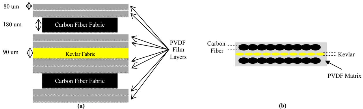
Figure 1. Schematic of the smart composite structure and material thicknesses (a) the stack-up of reinforcement fabrics and PVDF film layers before melting, (b) after melting.
