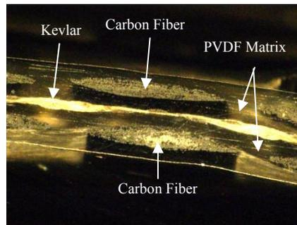
Figure 2. Cross section of the prepared samples.
