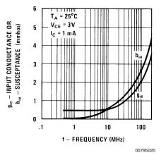
Typical Reverse Transfer Admittance vs Frequency
