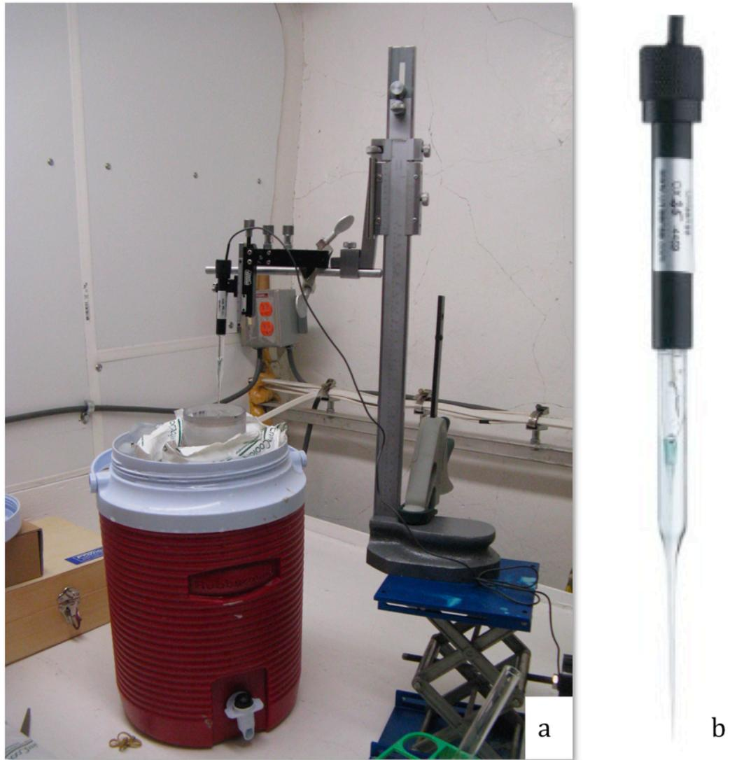
**Figure 5. a. Measurement of sediment oxygen concentrations; b. Unisence (Clark-type) microelectrode (Revsbech 1989)**
