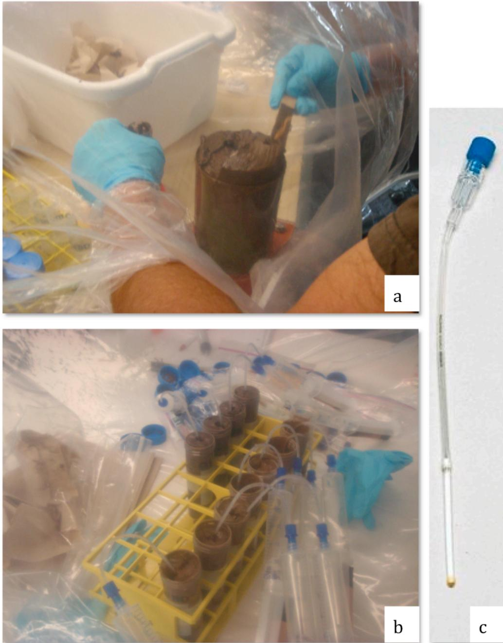
**Figure 4. a. Sectioning of a sediment a core in a glove bag filled with  $N_2$ ; b. Extracting sediment porewaters with Rhizon samplers in a  $N_2$ -filled glove bag; c. Rhizon sampler: hydrophilic porous polymer, pore diameter of  $0.1 \mu\text{m}$ . The fluid sampled from the sediment flows into the tiny space between the porous tube and the supporting wire.**
