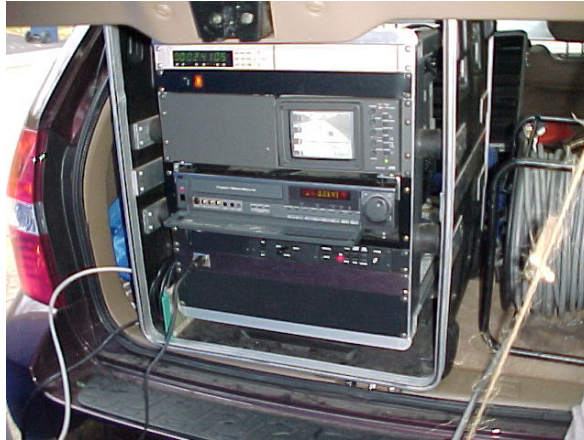
Figure 8: Video recording system with loop actuation and timestamp
