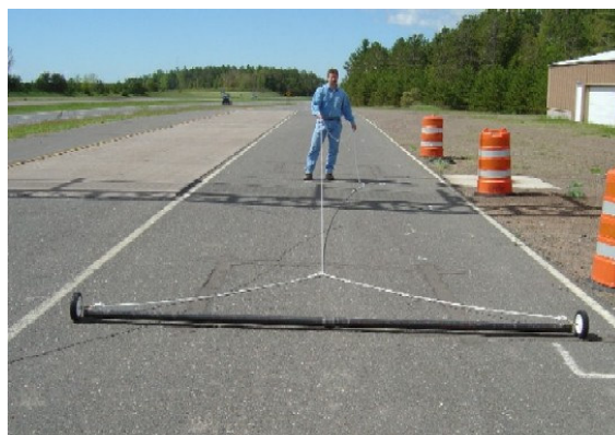
Figure 9: Apparatus used for loop system impulse response
