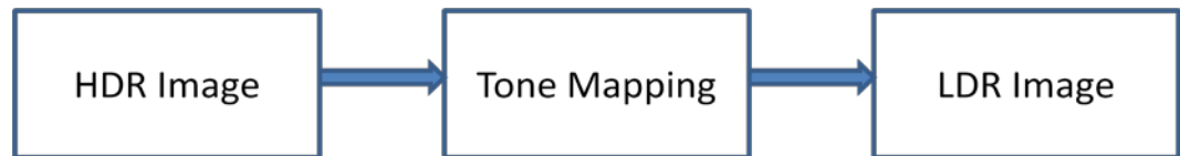
Figure 3.23 The whole scene is rendered using high dynamic range then tone mapped to convert it to low dynamic range in order to be displayed on the monitor.
